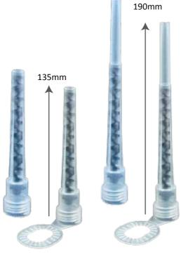
superior mixing compared to other mixers currently available. instantly mixed product with no wastage. x9 helical mixing deflectors inside. special disruptor for diffusion effect to reduce force.
