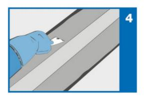
Once the second layer of **Adesilex PG4** has been applied, sprinkle on a layer of **0.5 Quartz** to create a rough surface and slowly remove the masking tape (fig. 5).
