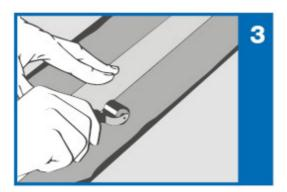
Apply a second layer of **Adesilex PG4** while the first one is still fresh, completely covering the fabric strip with the new layer of adhesive (fig. 4). Smooth off the product with a flat trowel.
