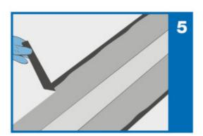
**Mapeband TPE** must be protected against damage (e.g. perforation) during the application process. If high levels of movement are foreseen, **Mapeband TPE** must be laid by forming an upside-down "W" (omega) shape on the inside of the joint (fig. 6).
