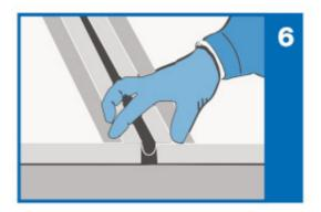
Butt joints between two strips of **Mapeband TPE** must be carried out by overlapping and bonding at least 5 cm of the central part in TPE by either hot-welding or cold-welding, as illustrated previously.
